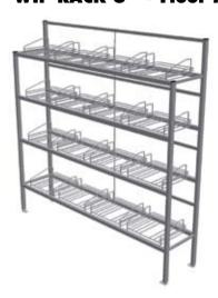
This WIP rack is suitable for 8" boxes and SMIF pods. Dedicated ports with integral signing allow easy identification, WIP identification system attachment is also possible. Minimal surfaces keep material clean and safe. Available in a variety of sizes. Fabrication material: 304 stainless steel, electropolished.
